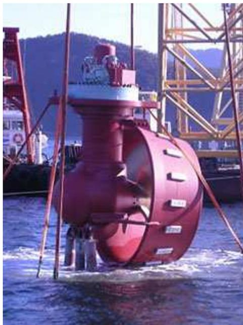
Figura 26 – Propulsor azimuthal
